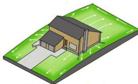
Ideal Water Runoff
